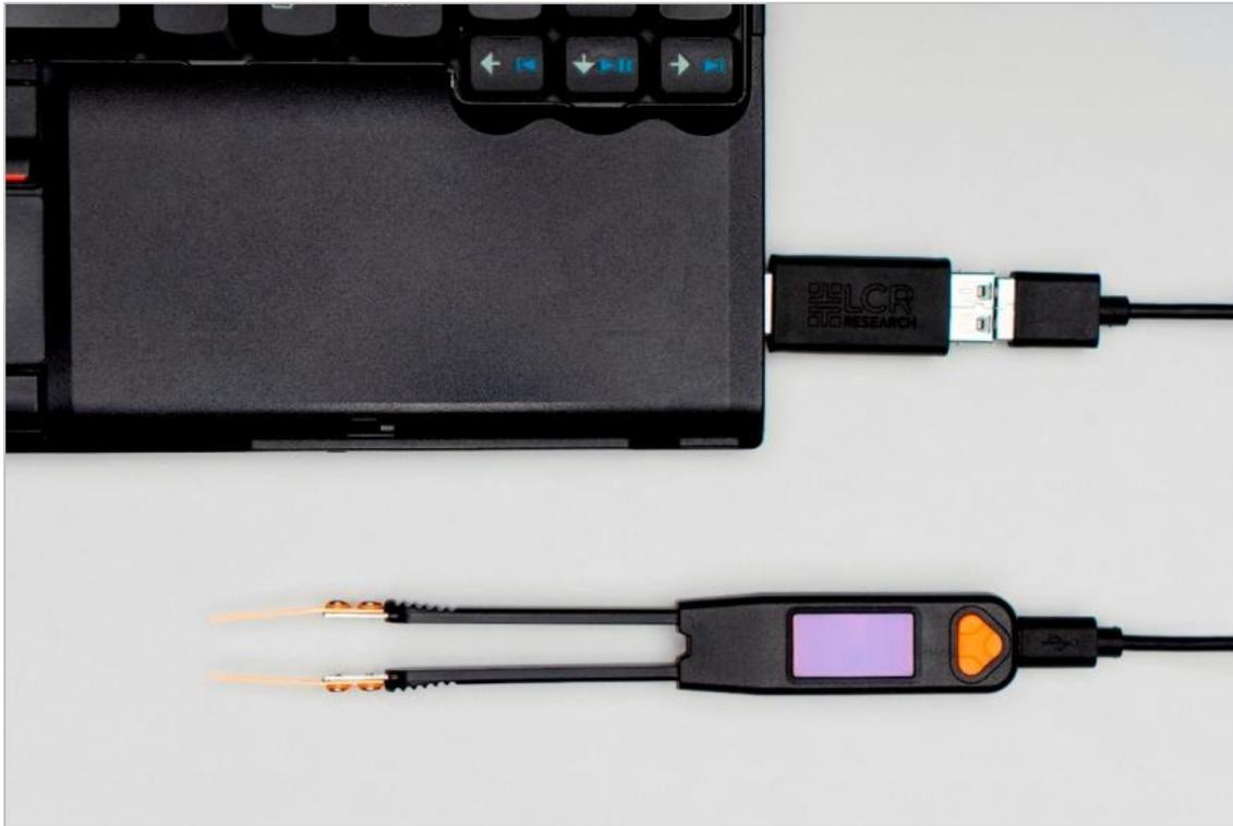
Figure 3-1: Connect LCR Pro1 to PC
